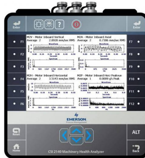
Figure 6: The Commtest vb5 and Emerson Process Management, CSI 2140 are typical portable data collectors available in entry level to advanced configurations (Photos courtesy of Commtest and Emerson Process Management)
