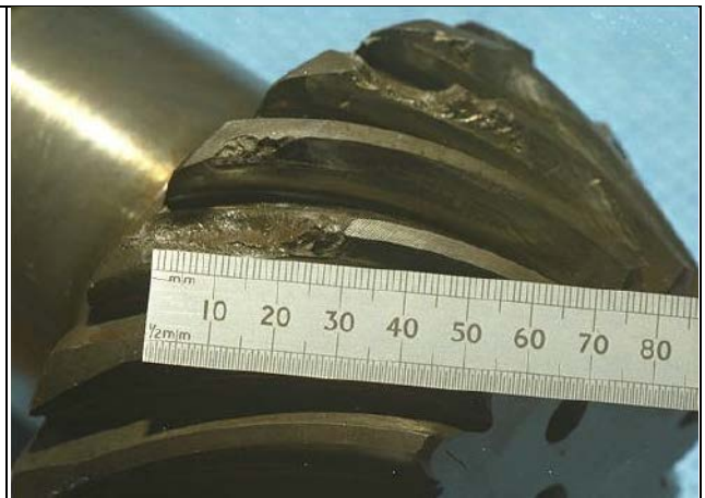
Figure 3(b) A broken Gear Box Teeth
