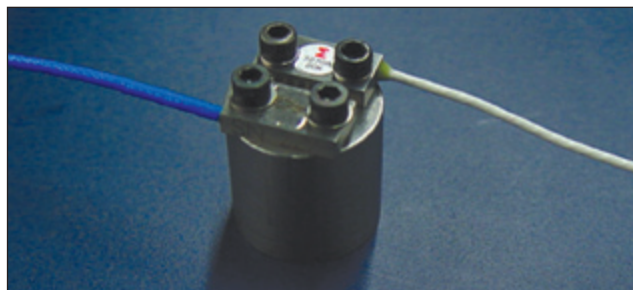
Figure 14. PCB and legacy shock accelerometer on breakaway fixture.
