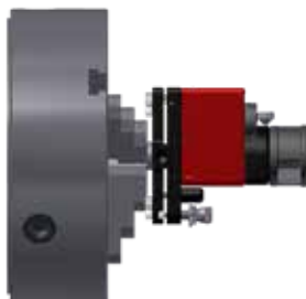
Use when measuring Straightness, Squareness and Spindle direction in a milling machine.
