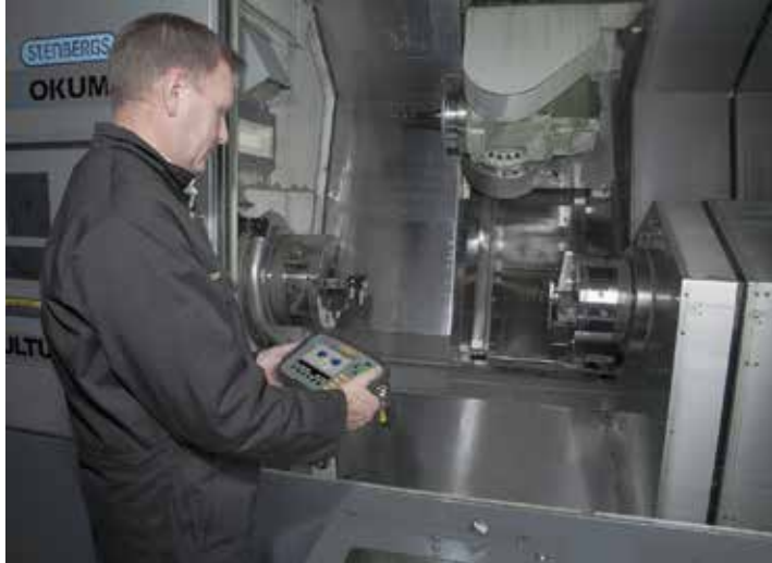
Easy-Laser® equipment mounted on a lathe with turret.
