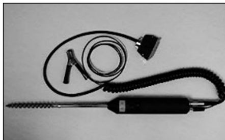
Figure 10. CSI Model 348SP Shaft Voltage/Currents Probe
